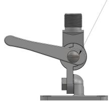
5: Tighten the lock nut by 10Nm while keeping the new handle position
