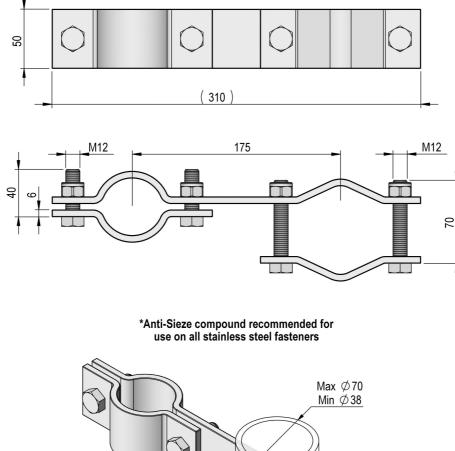
Fix the M12 bolts by max 9Nm Use collar supplied with the antenna (Do not use additional filler)
