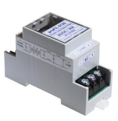
proFIL0120 removes interference from DC-power lines and protects sensitive communication equipment. It helps users to meet various EMC-standards. Proven performance specially with lighting, electrical drives and communication gateways.
