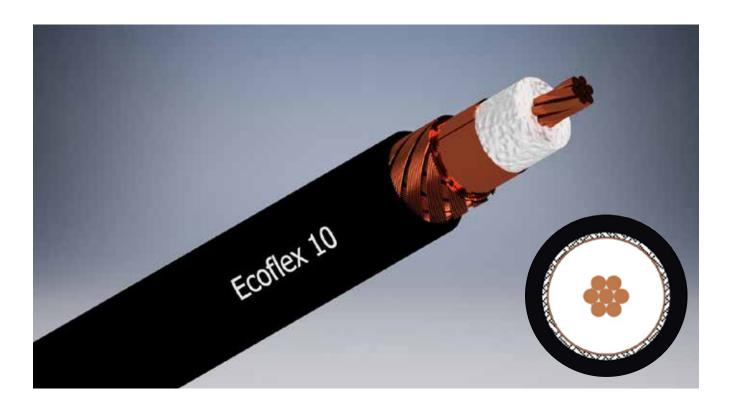
Ecoflex 10 is a flexible, low loss 50 ohm coaxial cable for the frequency range up to 6 GHz. Advanced manufacturing techniques combined with the use of a low loss PE-LLC dielectric with a foaming rate of more than 70% result in very low attenuation values, which set standards among flexible coaxial cables of this dimension.
